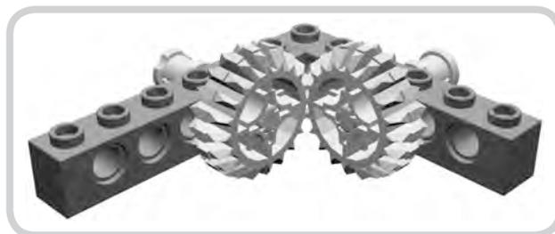
Figure 4-27: Here 20t double bevel gears are engaging on skewed axles.
