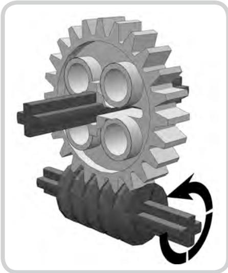
Figure 4-28: In this setup, a worm gear engages a 24t gear. The worm gear always rotates the other gear, not vice versa.
