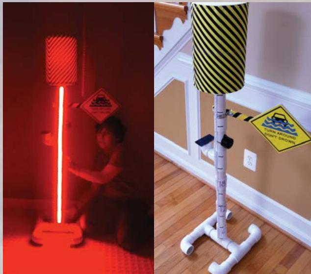
Our solution-the Automatic Staged Alert System (**ASAS**) uses flood water to trigger one of three driver warnings using motion, sound and light.
